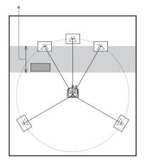
• You may not get the bass sound efficiently when the subwoofer is placed outside (③). You need to adjust the setting of the distance from the listening position.
